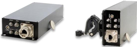
The PRE-226G-D-R contains two high performance RF front end modules covering the 2-26.5GHz frequency range. It utilizes state-of-the-art integrated circuit receiver technology and custom distributed circuit designs to produce a miniature RF front end. The module is packaged in a ruggedized, shielded aluminum case, providing a durable design suitable for field and portable use.
